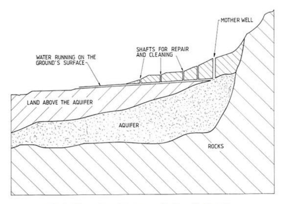
Fig. 2. Schematic vertical cross-section for a falaj in Oman.
