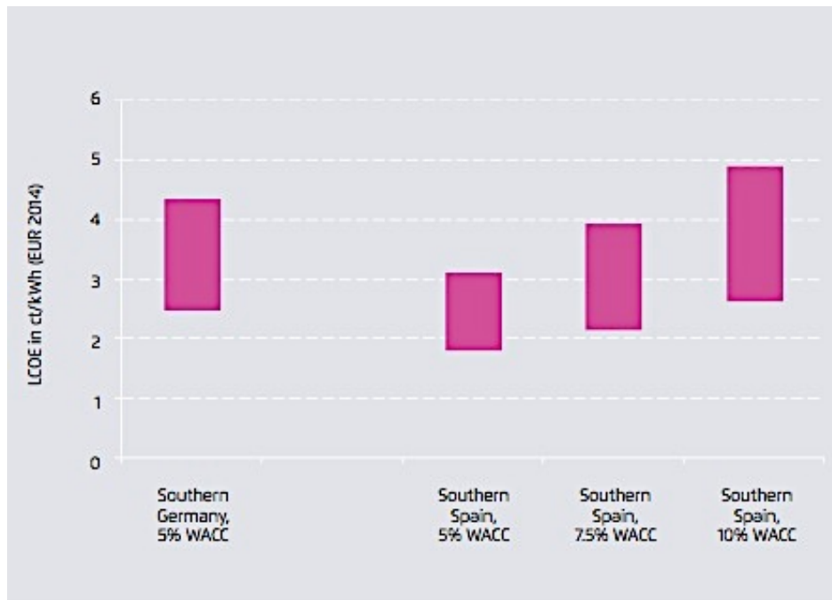
Figure 8: Range of Levelized Costs of Electricity Derived from Solar PV in Southern Germany and Southern Spain, based on Variable Capital Costs
